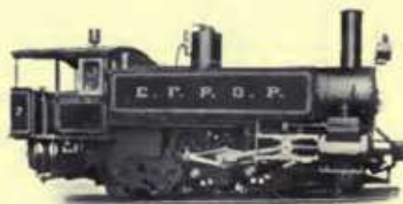
RACK LOCOMOTIVE WITH TWO COG-WHEELS
